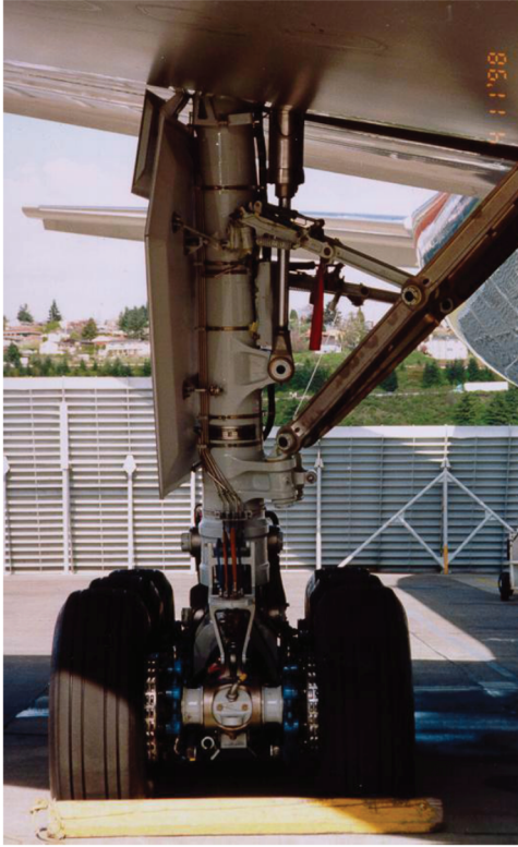
Fig. 2 Photograph of the main landing gear of the Boeing 777 aircraft.
